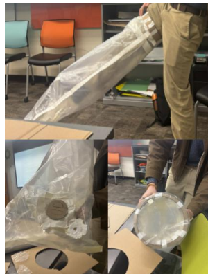
Figure 3: Low-fidelity prototype and key functional components, including mock-ups of the screw-cap and vacuum splint port
