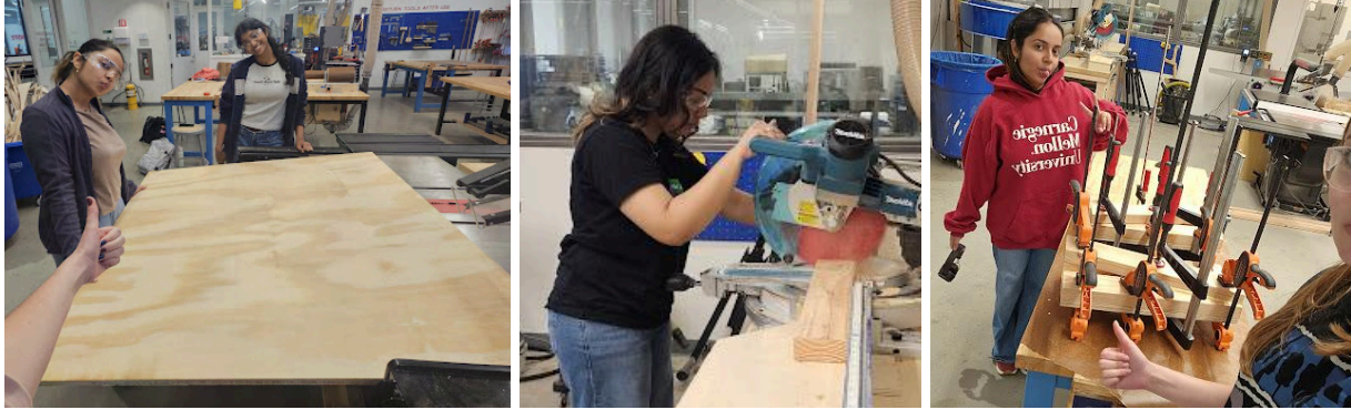
Figure 10.16. Left & Center Images: Cutting lumber for assembly of the backboard. Right Image: Gluing and clamping pieces of wood together to create supports for the acrylic reservoirs.
