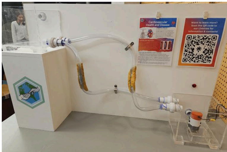
Figure 10.15. Fully assembled Stent Demonstration Model before being filled with simulated blood.
